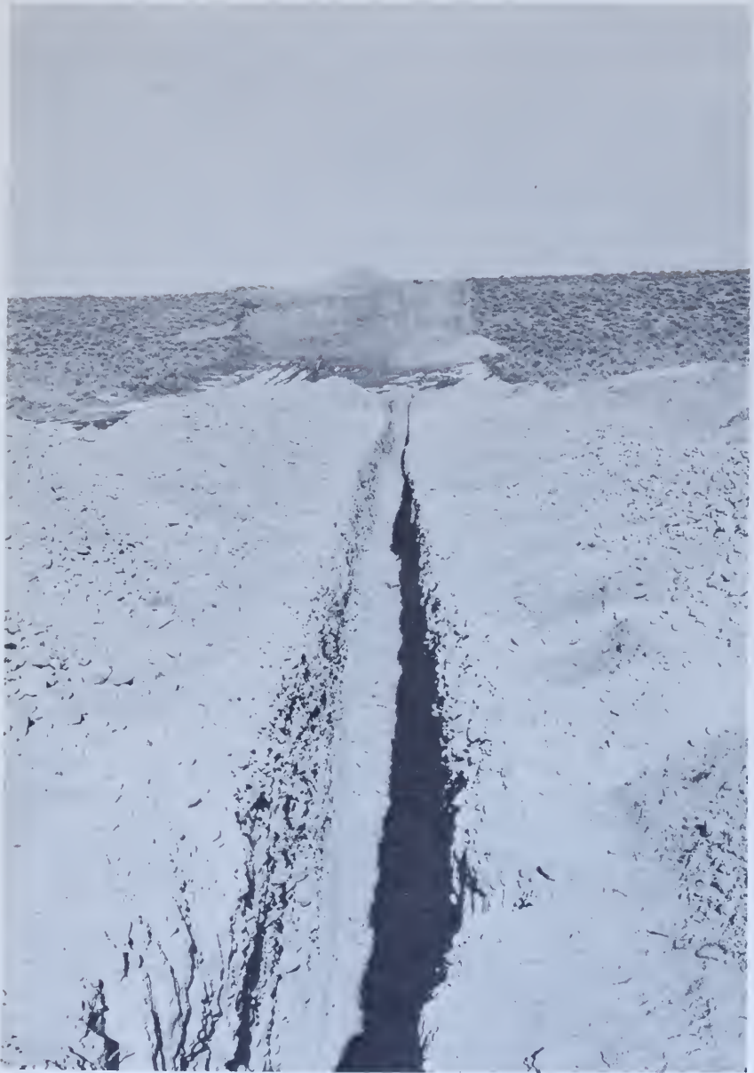
Figure 48.—Trench in Henrys Fork aggregate deposit, Flaming Gorge unit, Utah. P591-421-1228.
